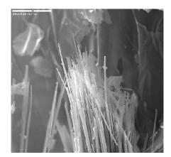
Scanning electron micrograph of asbestos fibers. (Photo: U.S. Geological Survey/U.S. EPA)
